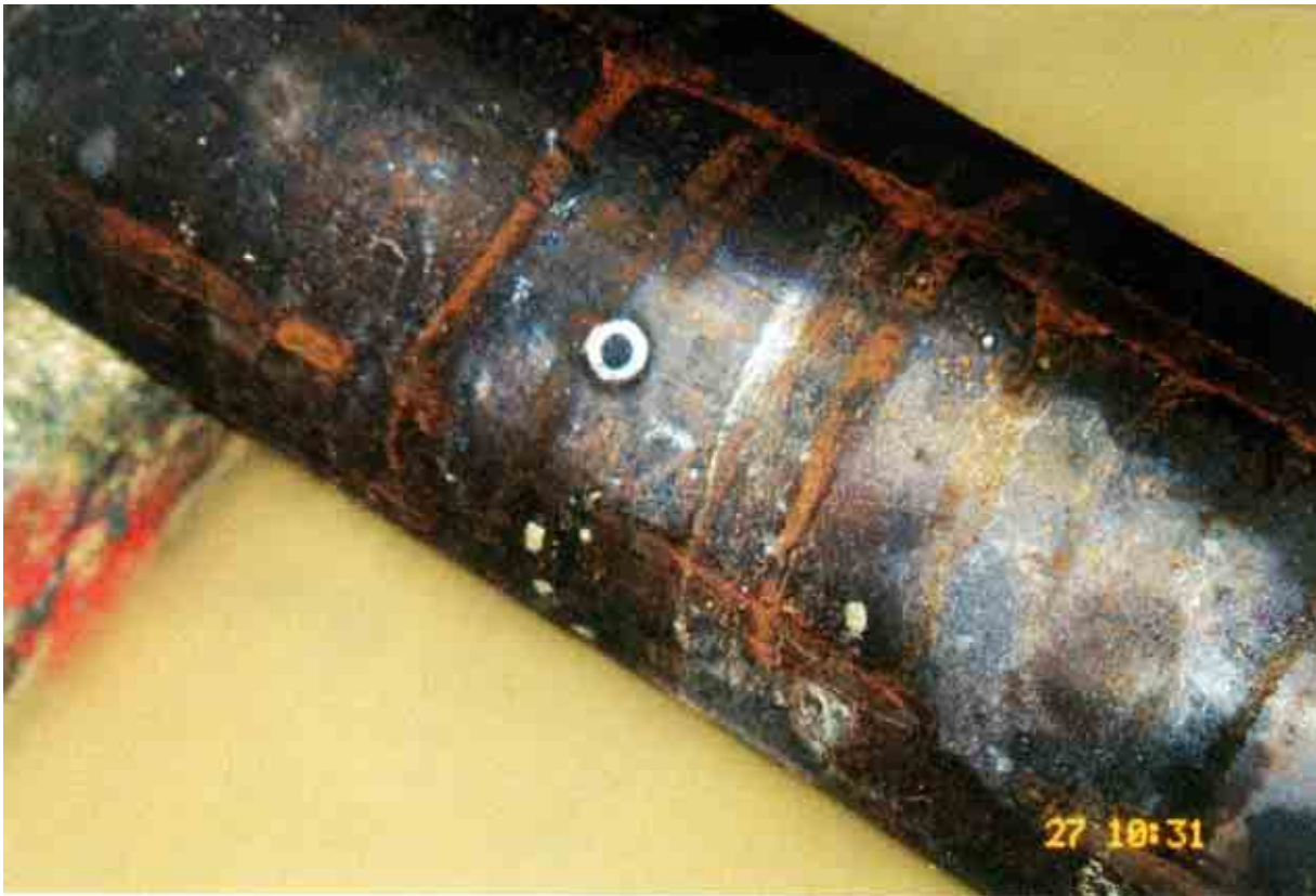
Fig. 2.32: Pipe with injection valve
