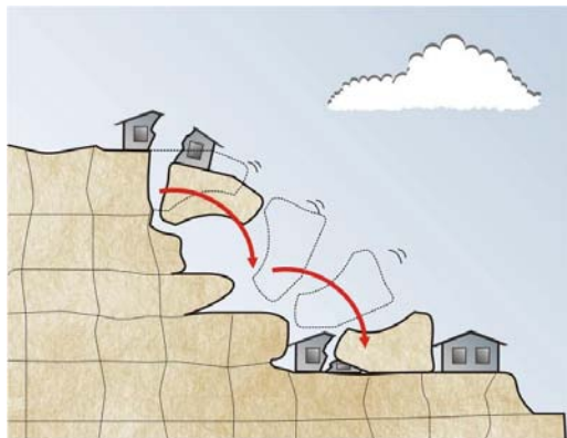
Figure 1 - Failure of an undercut block
